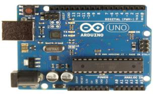
Figure 5: Arduino ATmega 328
